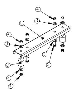
Sub-Frame Assembly (V-Twin Engines)
